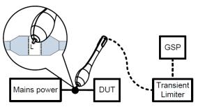
PR-02 is an EMI electric field probe, which can maximally sustain CAT I 50V DC. PR-02 electric field probe will
