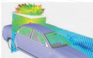
Automotive application: 2.45 GHz antenna on top of a car. Electric field and far field pattern.
